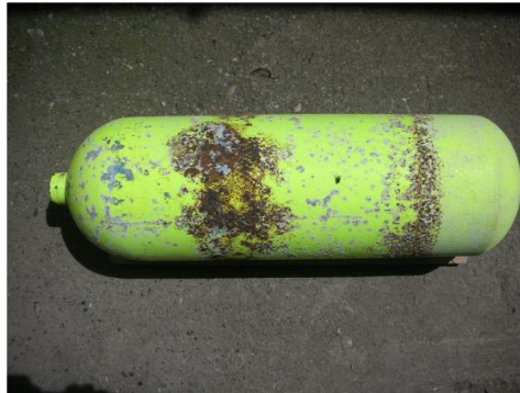
Fig.19. TO TAKE CARE OF YOUR DIVING EQUIPMENT AND TECHNIQUE IN THE NEW YEAR: Spongy electro-corrosion of the bottle.
