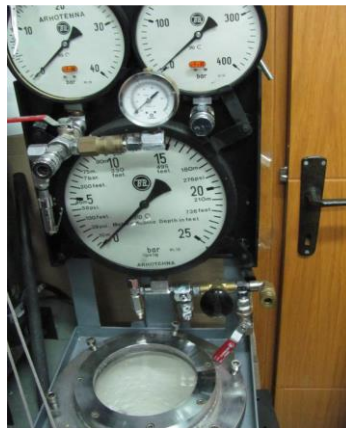
Fig.20. YES FOR THE SERVICE OF DIVING EQUIPMENT AND TECHNIQUES YOU HAVE: Enough instruments - Chamber for checking the operation of the regulator in water under depth pressure.
