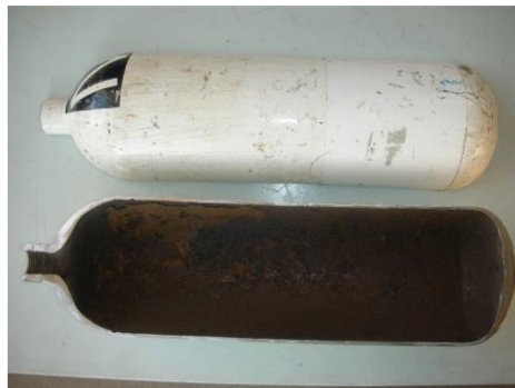
Fig.17. TO WATCH YOUR DIVING EQUIPMENT AND TECHNIQUE IN THE NEW YEAR: Spongy corrosion of the inside of a small bottle.
