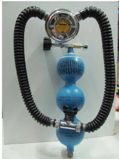
Fig.42. To use breathing equipment and techniques used in aviation for diving. - From the Diving Equipment Museum of this Club. Oxygen bottle for Russian jet planes flying at high altitudes.
